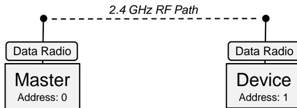
When using a RF data radio module instead of a wired connection, the logical behavior is exactly the same. Data that comes out of the master’s UART will arrive at the input to the UART on the slave.
